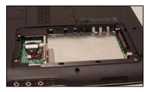
If your hard drive attaches to your motherboard via a cable, hold the cable's connector - not the cable itself - and gently remove the drive from it.
